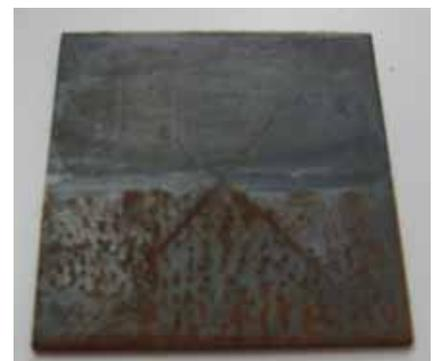
**Passes 250 hours of Salt Spray Test**
